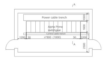
Figure1:plane diagram for switchgear arrangement scheme
