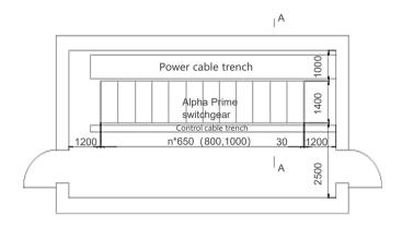
Figure1:plane diagram for switchgear arrangement scheme
