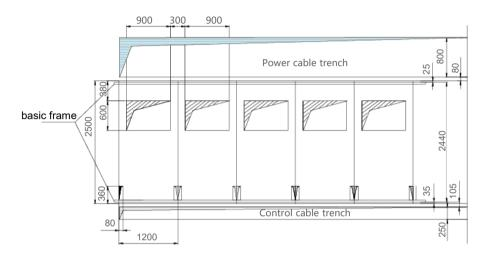
Figure3:Switch-room cable trench arrangement scheme
