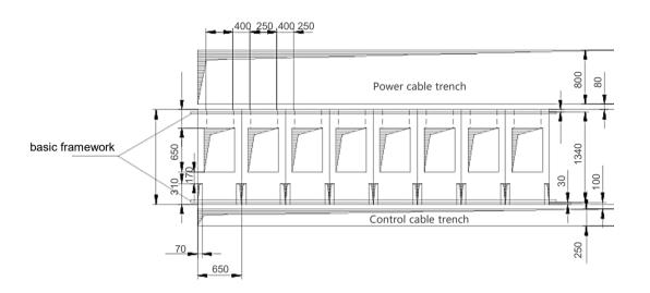
Figure3:Switch-room cable trench arrangement scheme
