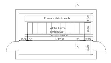
Figure1:plane diagram for switchgear arrangement scheme
