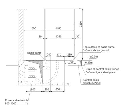
Figure2:plane diagram for switchgear arrangement scheme (section A-A)
