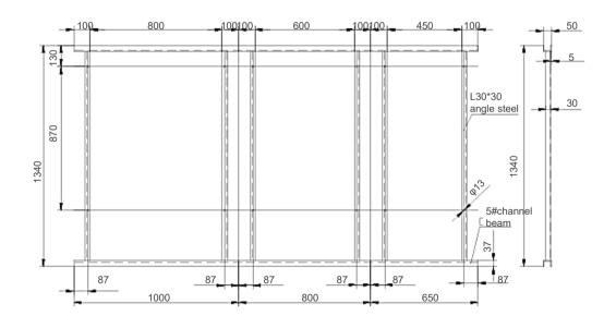
Figure4:Typical basic frame foundation (for 1000mm/800mm/650mm width dimension model)
