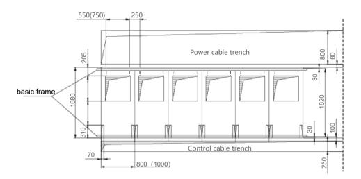
Figure3:Switch-room cable trench arrangement scheme
