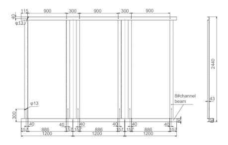
Figure4:Typical basic frame foundation
